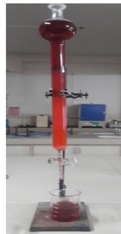
Figure 2: Column chromatographic purification of the prodigiosin solution, this process enhanced the removal of the excess extracting solvent and separated the pure PG from other contamination agents.
