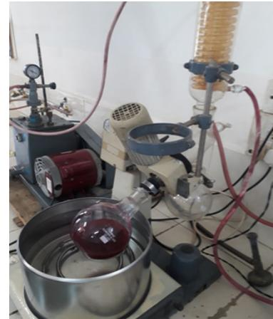
Figure 1: The concentration by rotary evaporation.
